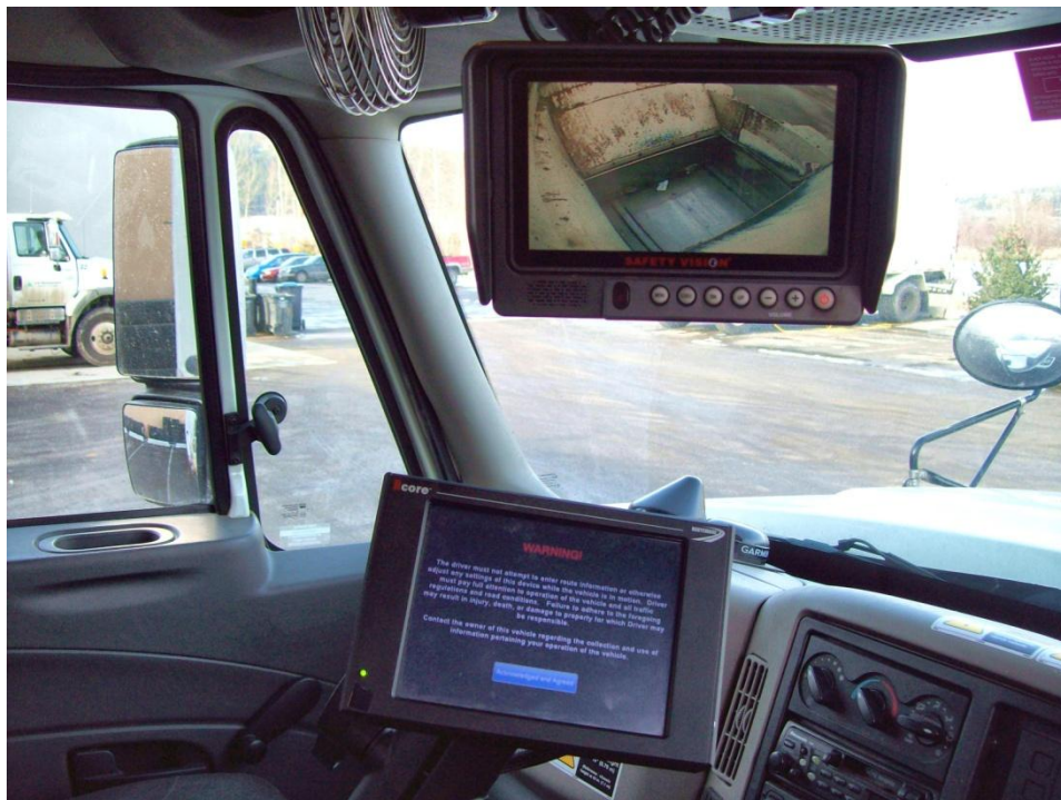
Cab of automated waste collection truck showing part of RFID software and monitor view of hopper.
