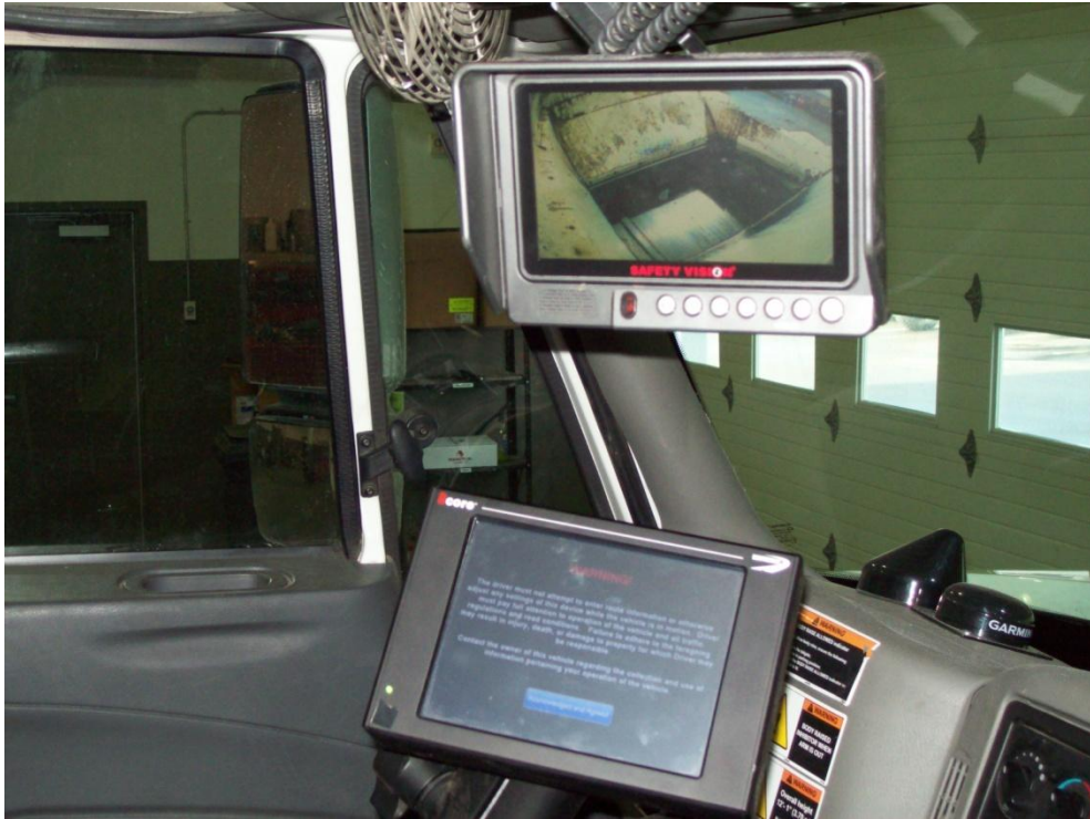
Cab of automated waste collection truck showing part of RFID software and monitor view of hopper.
